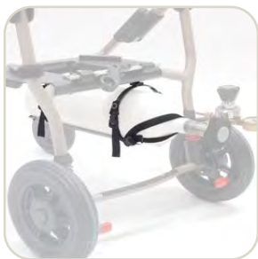
935 Oxygen bottle holder. Maximum dimensions of the oxygen bottle: height 600 mm (valve included) – diameter 140 mm. For 869 base the frame can be folded without removing the accessory
